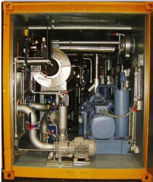
40 ft container with CO<sub>2</sub> / NH<sub>3</sub> soil-freezing containerised refrigeration system
