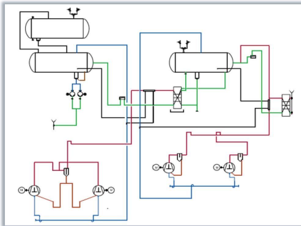
Schematic PI-diagram of the CO<sub>2</sub> / propene-cascade refrigeration system
