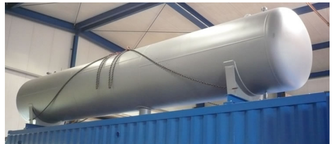
Ready-to-ship explosion-proof CO 2 / Propane cascade refrigeration system at the manufacturer's plant in Sörup
