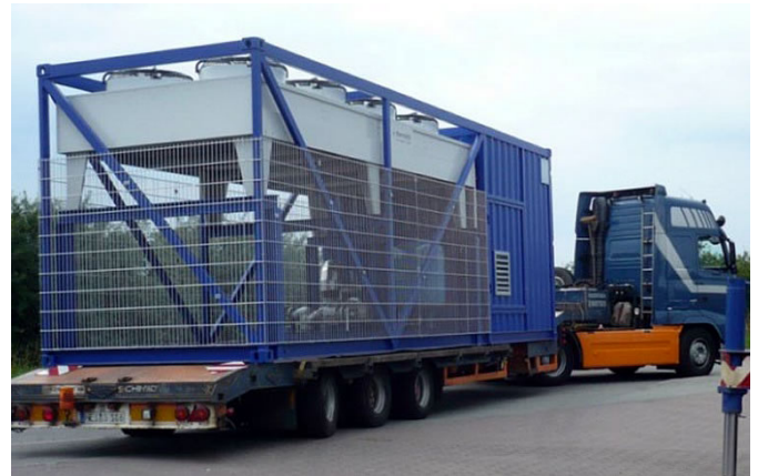
Mobile NH 3 Refrigeration System
