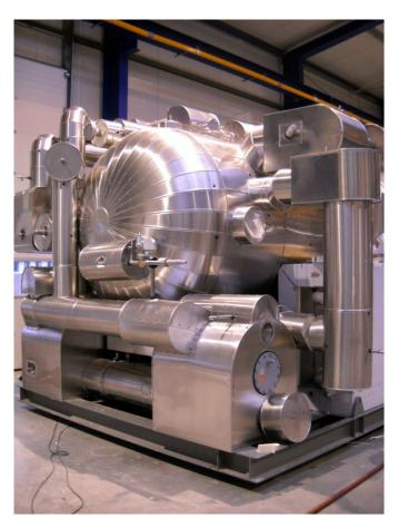
$\rm NH_3$  / R23 Cascade Refrigeration System for Cooling Toluene to -20.5° C, -53.5° C, and -70.5° C
