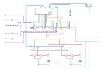
To achieve the low evaporation temperature, the NH3 screw compressors are designed in a 2-stage configuration.
